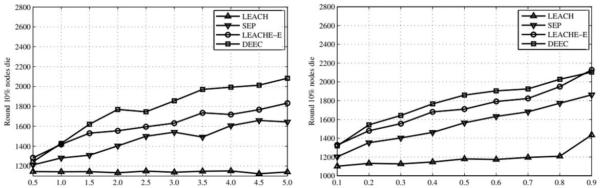
Fig. 5. Round 10% nodes die when  $m$  and  $a$  are varying.
