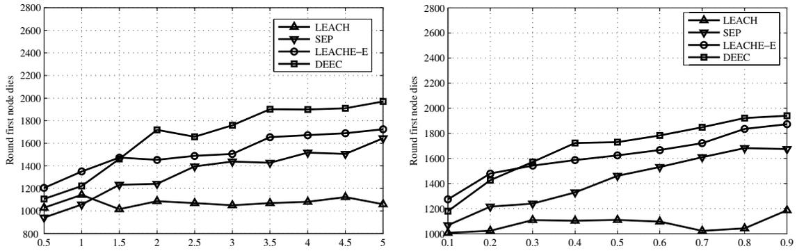
Fig. 4. Round first node dies when  $m$  and  $a$  are varying.
