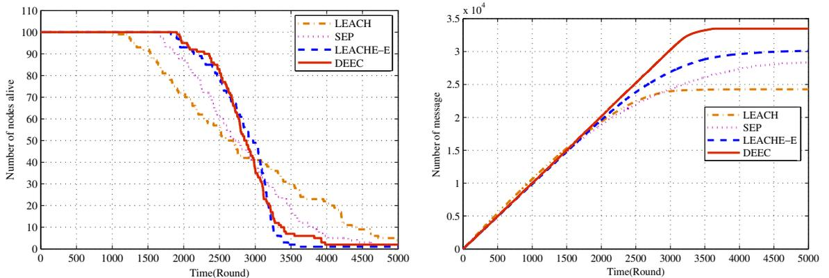
Fig. 6. Performance of LEACH, SEP, LEACH-E, and DEEC under multi-level heterogeneous networks. (Left) Number of nodes alive over time. (Right) Number of message received in base station over time.
