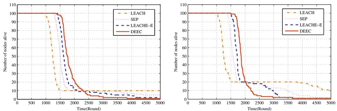
Fig. 3. Number of nodes alive over time of LEACH, SEP, LEACH-E, and DEEC under two-level heterogeneous networks. (Left) When  $m = 0.2$  and  $a = 3$ . (Right) When  $m = 0.1$  and  $a = 5$ .
